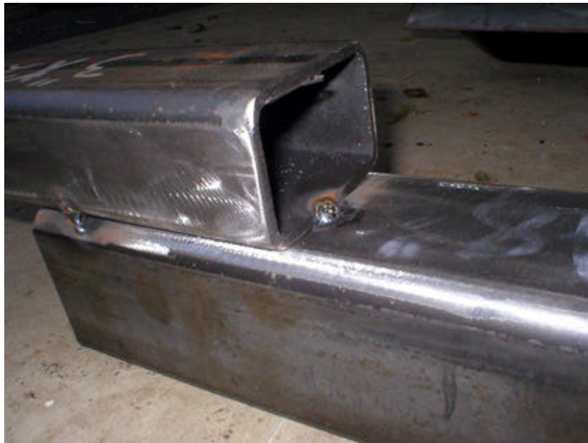
Outriggers tacked in place. On a structure like this, it is critical to get a good weld on every single surface you can reach.
