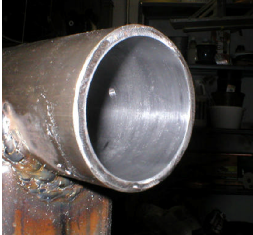
Inside of rotator sleeve is smoothed to help make rotation easier. Also note the hole for the grease fitting.
