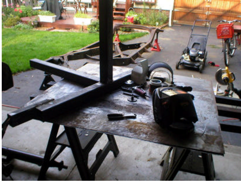
Setting work up at a comfortable level leads to quality welds.
