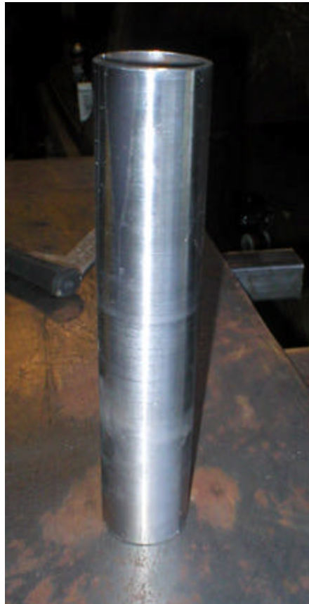
Turning the pin diameter down slightly made it fit perfectly in the sleeve.
