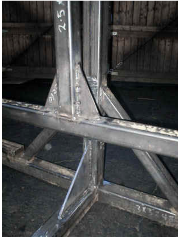
Triangular gussets add strength without taking up too much space on the horizontal bar.
