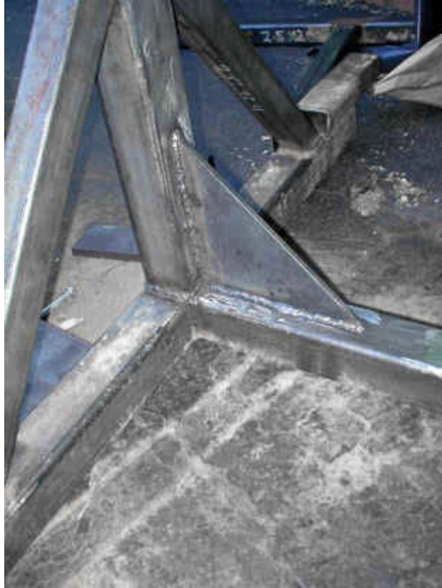
Plate steel gusset does the job just fine.
