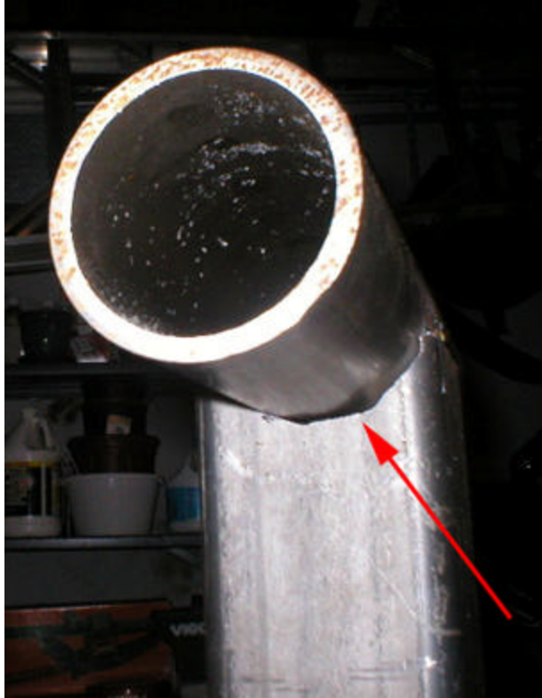
Carefully cut your cradle area. Note that the cradle is not quite equal to the radius of the rotating sleeve.
