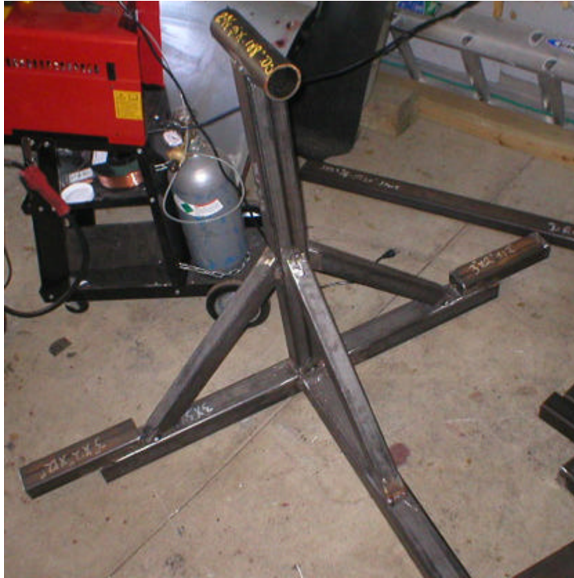
All 3 diagonal braces meet at the same height, indicating that the upright is perfectly square to the base.
