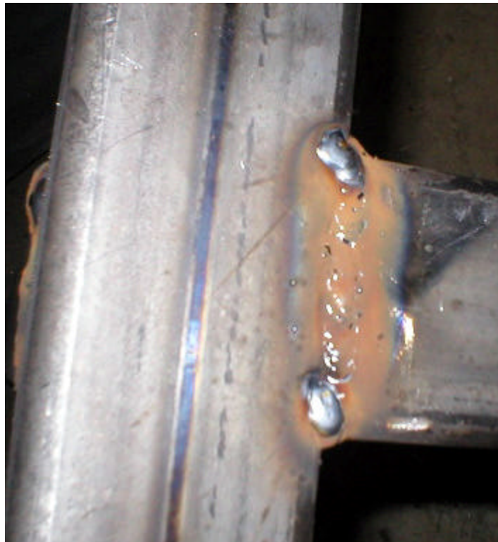
Another decent weld. Corners are thicker because of passes from each side and the back overlapping.
